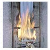
EN 50266-2-4:2001 / BS EN 50266-2-4:2001 / DIN EN 50266-2-4:2001 / VDE 0482-266-2-4:2001-09 / CEI EN 50266-2-4:2001 — Common test methods for cables under fire conditions. Test for vertical flame spread of vertically mounted bunched wires or cables - Part 2-4: Procedures. Category C (Replaced by EN 60332-3-24:2009).
